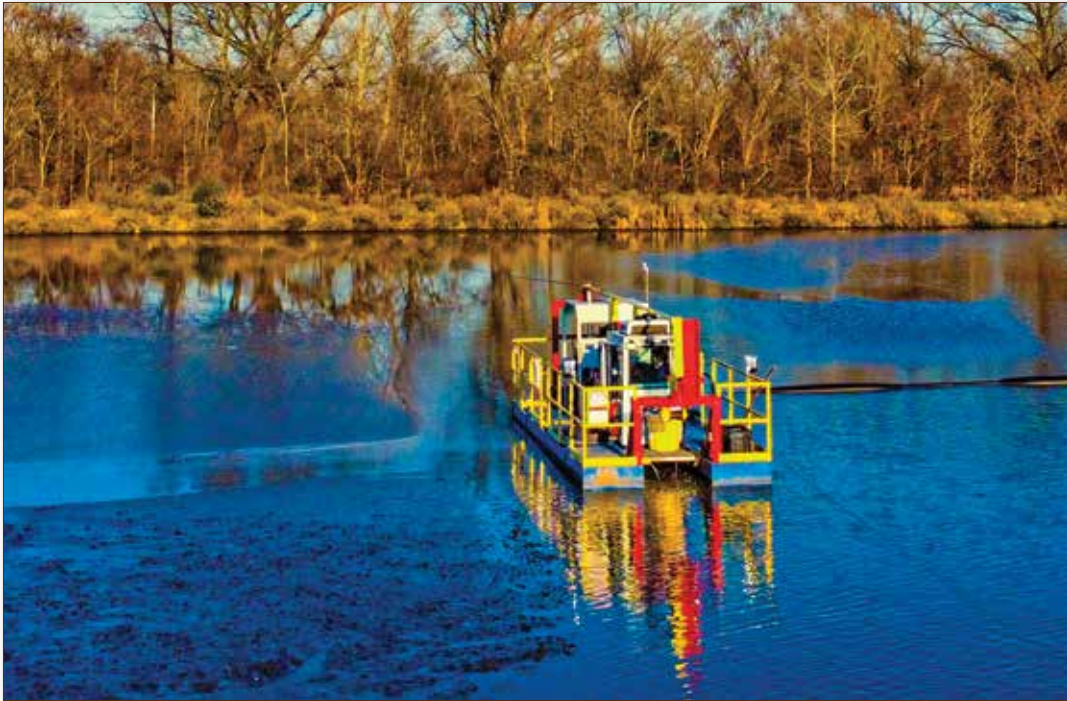
Eagle's Mud Cat 115D systematically cuts parallel rows using its 4-point cable drive propulsion system. Note the heavy solids at the left of the photo.
