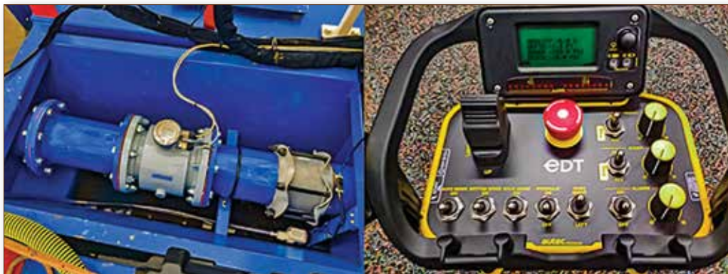
Mud Cat's Flow Sense gives the operator real-time pump flow measurements from the convenience of a digital gauge in the climate-controlled cabin.
