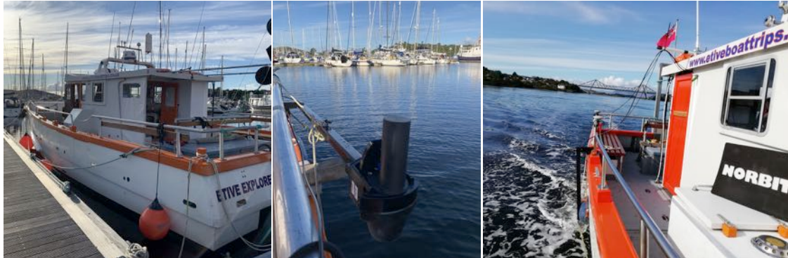
Survey vessel and hardware installation on an over-the-side mount.
