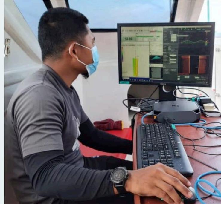
Real time positioning was obtained using Marinestar G2 DGNSS signal directly injected into the POSMV OceanMaster module. Positional data was further enhanced in post processing using Applanix PP-RTX solution and depth are based on EGM96 Geoid Model.
