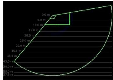
*Real time GUI display - electronic steering is employed to image vertical structures*
