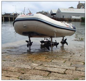
The craft employs a fully automated retractable MBES transducer mount and is fitted with an Applanix POS MV inertial navigation system for highly accurate survey control. It has been deployed with the highest resolution sonars and lasers available, having been mobilised with full size Reson and R2Sonics multibeam systems. Gimbal stabilised 4K stills and video cameras provide a visual record of the asset.
