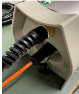
Figure 12. Power cable correctly connected to PDC.
