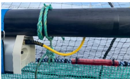
Figure 7. Correct curve on cable
