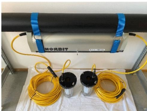
Figure 1. One PDC powers two 600-watt lamps
