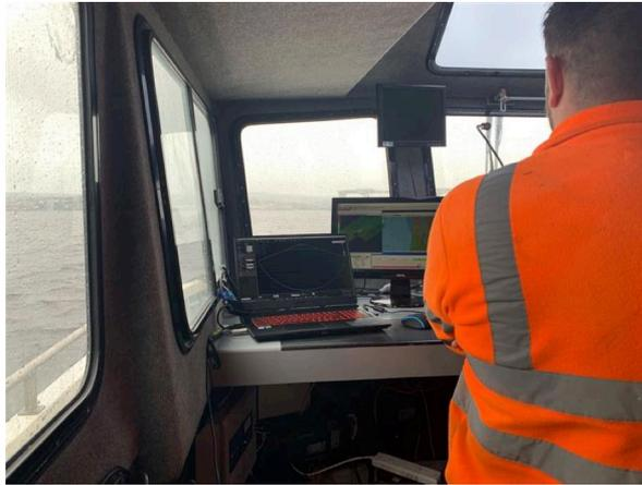
*Surveyor station in cabin with laptop control for NORBIT and HYPACK*
