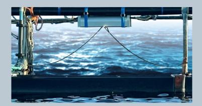
From the PDC comes a fixed cable on the right and left side respectively. These cables are attached to the handrail with two accompanying Velcro bands, which then forms an additional safeguard against the device coming loose. Weighing only 17 kg, the unit is designed to be lightweight in order to facilitate assembly and avoid possible damage to the handrail.
