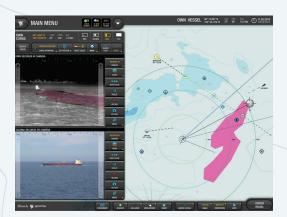
The SECurus is the most important sensor when fighting oil spills, with the ability to estimate relative thickness and volume of an oil slick. Every pixel in the video is georeferenced.
