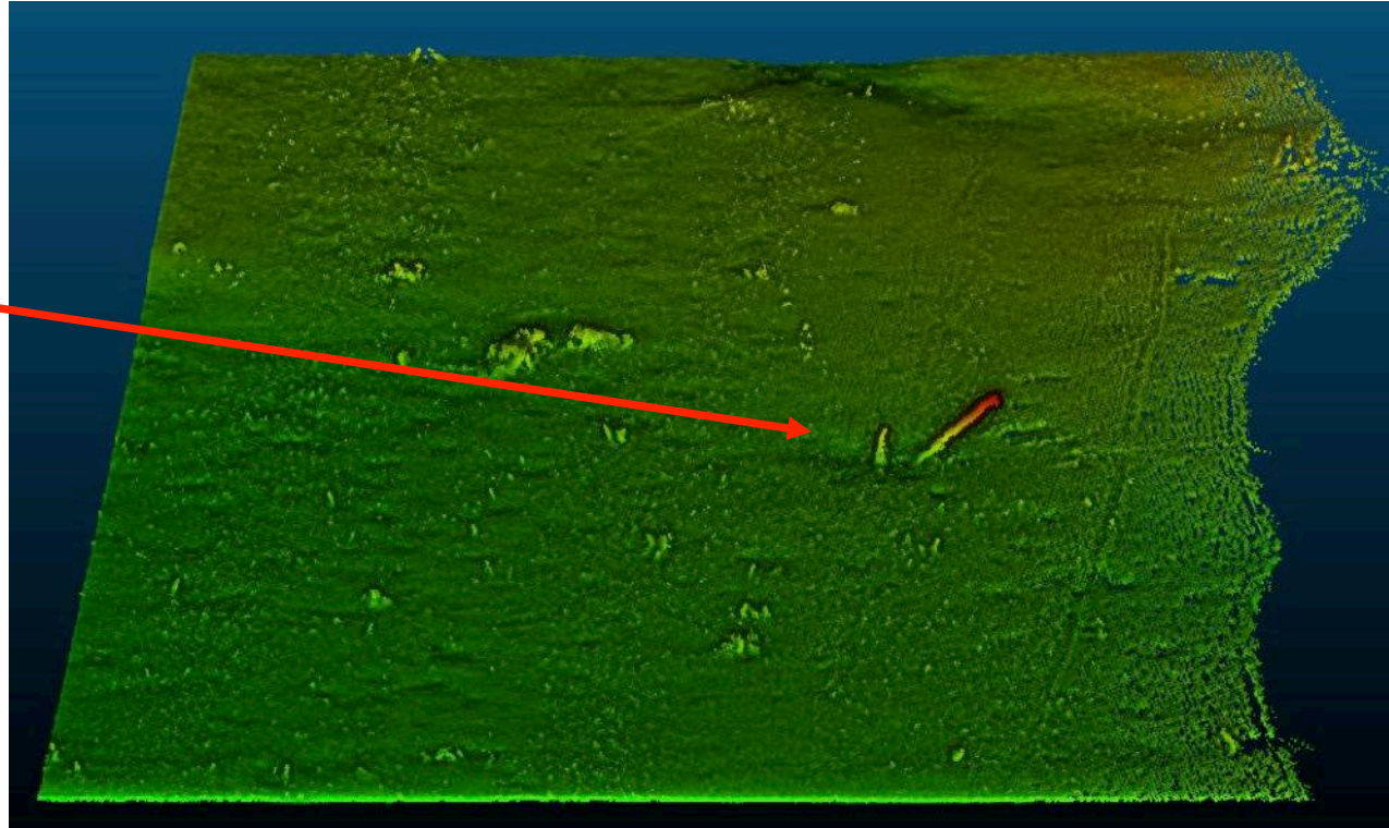
Kedge-Admiralty type anchor shown in processed full resolution point cloud, shading and illumination applied
