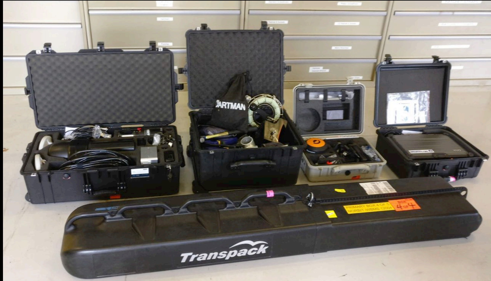
Full survey kit, Sonar, INS, mount, base station and PC. All items can be checked in Airline luggage
