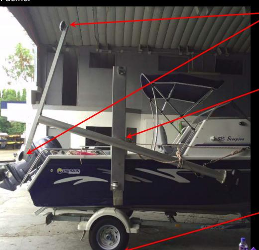
Antennas fixed to sturdy antenna bar 2 meters apart.
