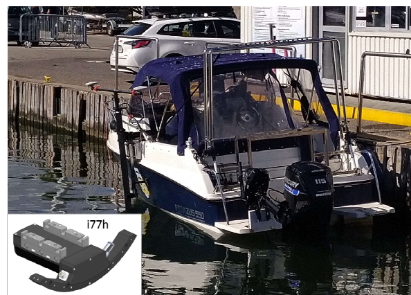
Fig. 2. The motorboat with the T shape pole mounted on the port side. In the left corner WINGHEAD i77h multibeam drawing.
