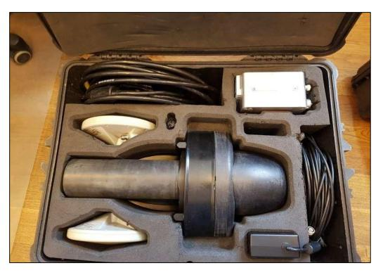
The NORBIT iWBMSh was identified as the ideal tool for the task, being both highly compact, as well as a highly specified, turn-key ultra-high resolution multibeam survey system.
