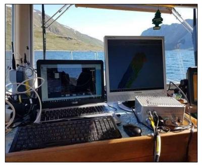
The iWBMSh was mobilised onto the Targa 25.1 alongside the Naval bases jetty., Grønnedal. The iWBMSh head and GNSS antennae were pole-mounted just aft of the wheel-house saddle clamped over the gunwales and secured to the railings. The NORBIT SIU, acquisition computer and helmsman monitor were set up on the chart table to the left of the cox's station in the wheel-house and the whole system was powered off domestic sockets by the boats own inverter supply.
