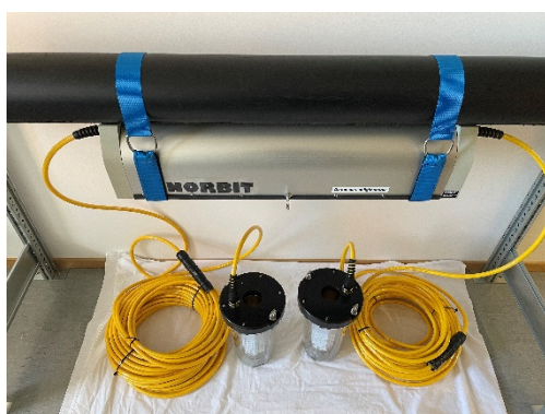
Figure 1. One PDC controls two 600-watt lights
