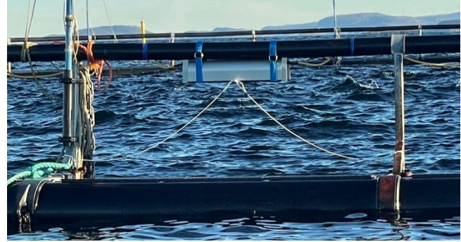
Figure 4. PDC mounted on the handrail with secondary protection.
