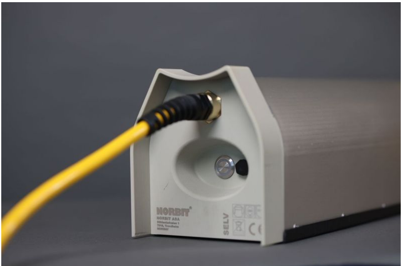
Figure 12. On/off button (silver coloured). The black "nut" is for pressure equalization and should not be touched.
