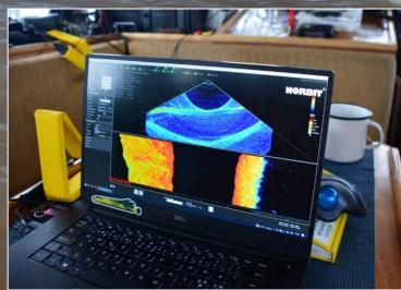
The light-weight and compact NORBIT WINGHEAD i77h multibeam and iLidar were easily adapted and configured for the use from the USV.
