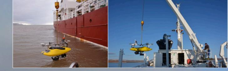
The WINGHEAD multibeam and iLidar in combination, mounted on the USV, were acquiring highresolution data at the calving glacier margins while the operator observed the incoming data quality and adjusted the survey parametres on the vessel at a safe distance over a WiFi link.
