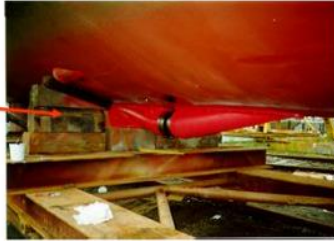
RESON SeaBat 8101 with fabricated for-and-aft conical fairings
