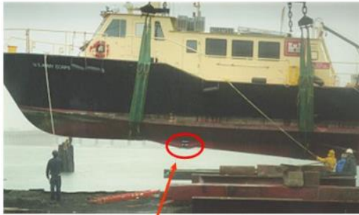
RESON SeaBat 8101 with fabricated for-and-aft conical fairings
