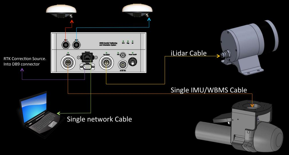
The integrated Norbit systems combines all sensors into a single small topside box. Power can be provided via AC or 12v battery. All systems connect to the survey computer via a single standard network cable.
