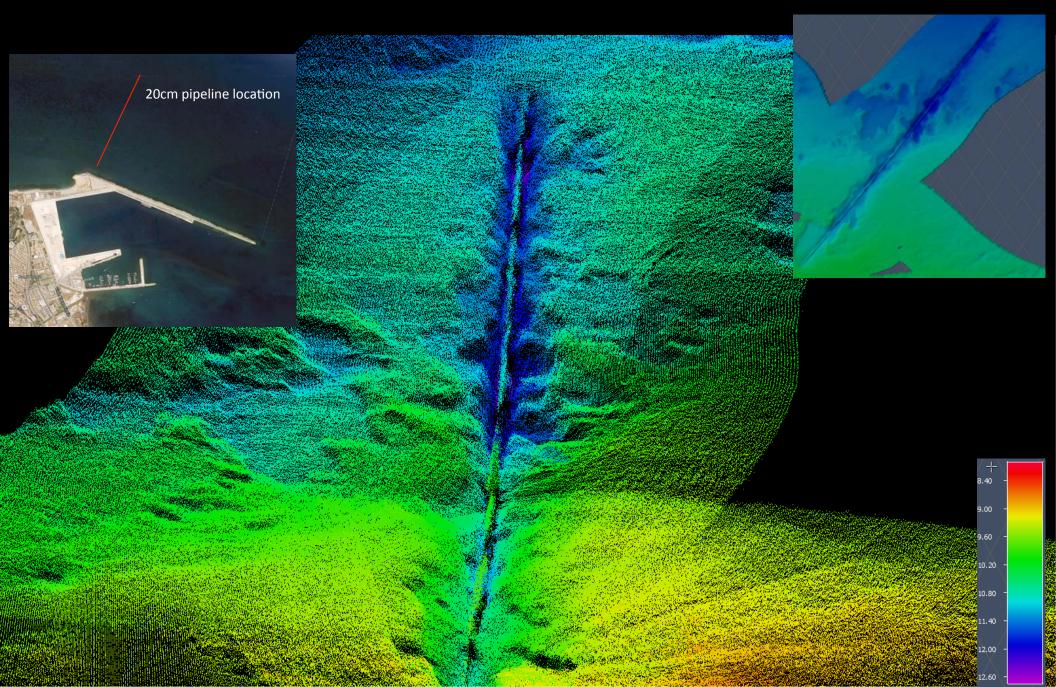
Profile over the pipeline – 700kHz
